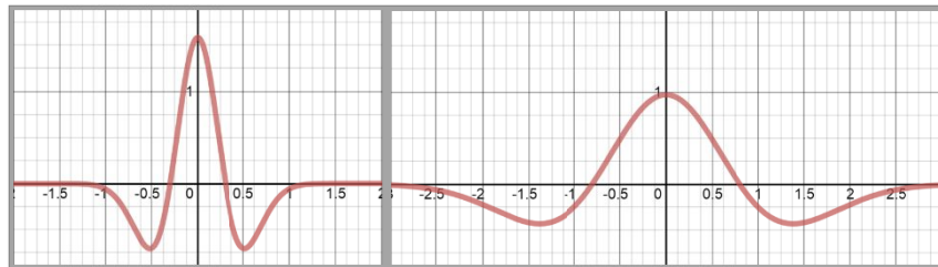
Figure 1: Mexican hat wavelet function in one dimension with scaling factor \sigma adjusted to .3 and .8 respectively.
